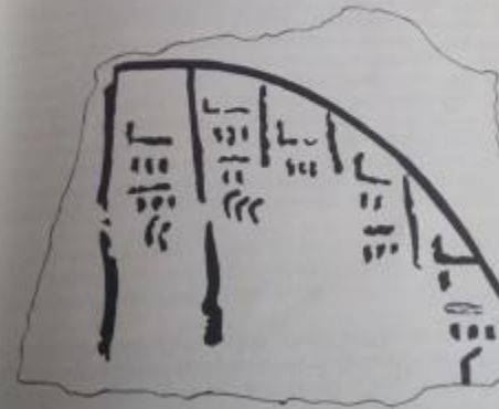
An architect's diagram, defining a curve by co-ordinates. Probably III rd dynasty, Sappara. Lumpkin — Fig.
