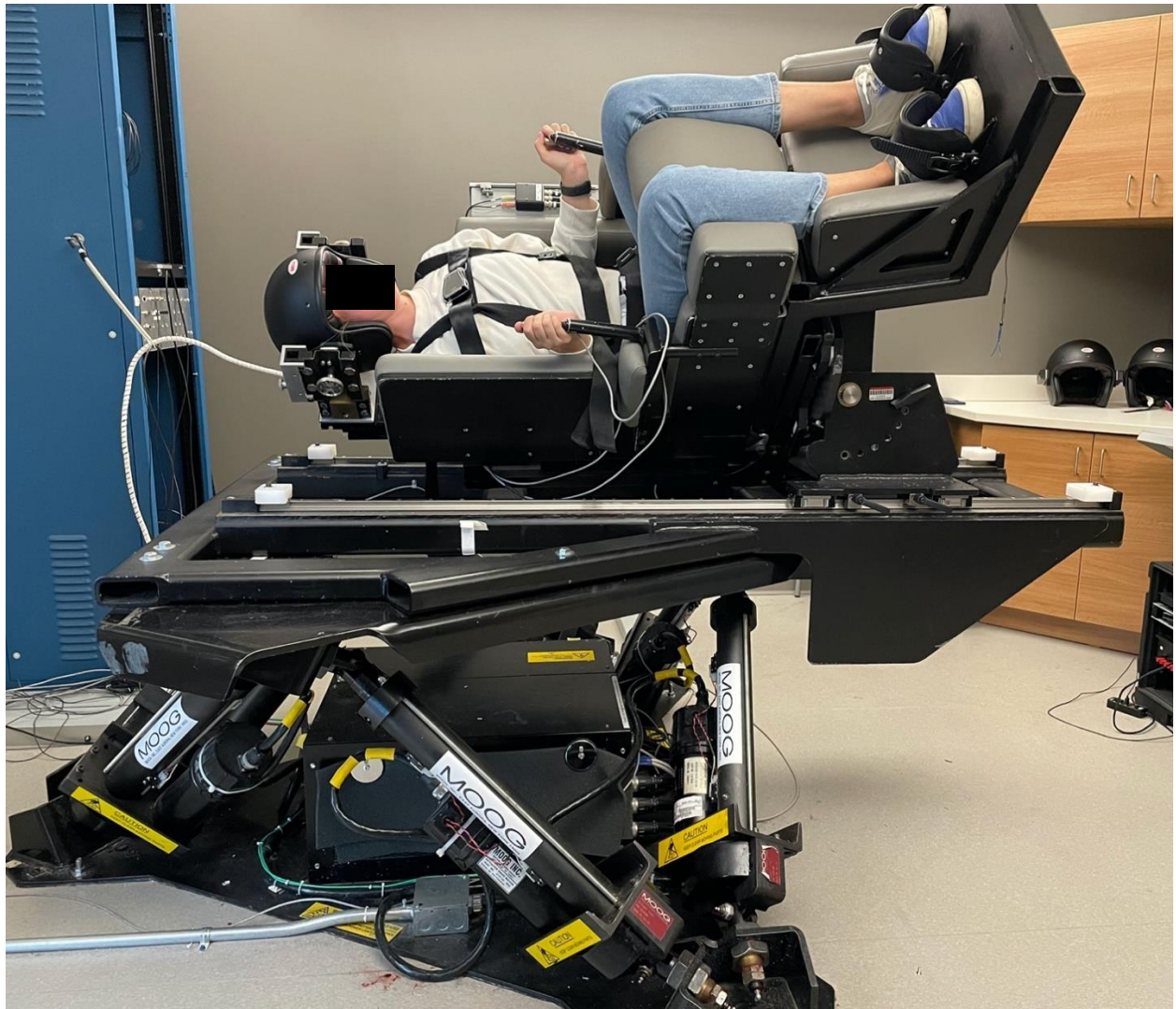
Figure S4. Chair is tilted backward 90 degrees and rotated 45 degrees to the right of supine. Earth vertical RALP rotations were delivered by rotating the subject about an earth vertical axis aligned at the level of the vestibular labyrinths (i.e., head-centered).
