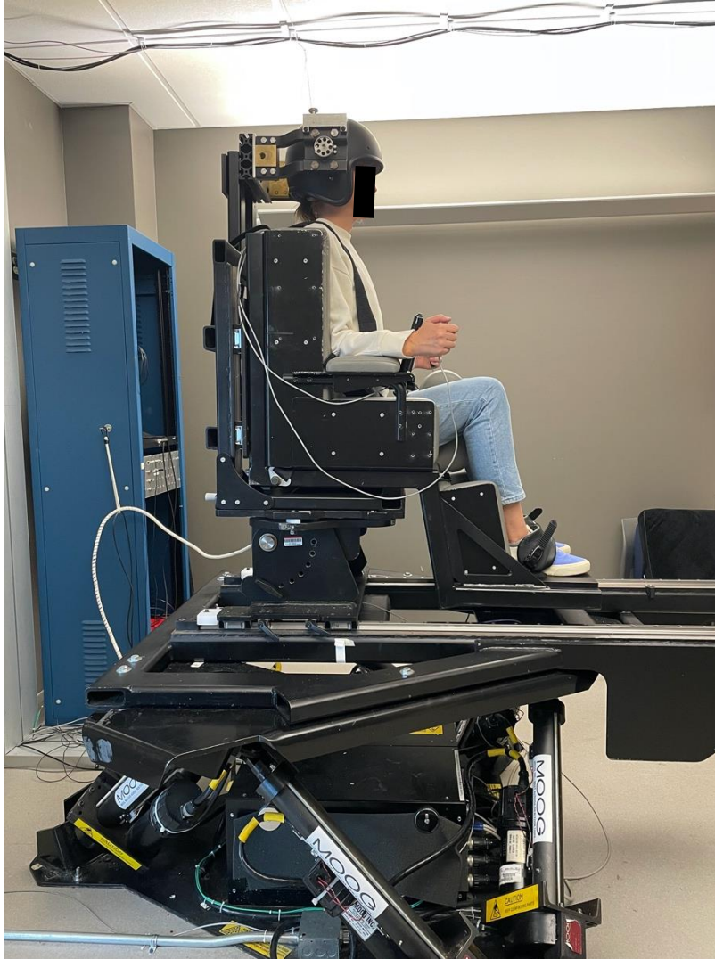
Figure S5. Chair remains upright for each of the Earth-Horizontal rotation (i.e., tilt) conditions. The MOOG 6DOF motion platform simulates the respective axes to permit head centered tilts in each of the respective motion planes.
