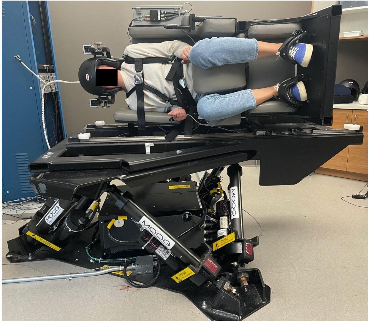
Figure S3. Chair is tilted backward 90 degrees and rotated 90 degrees to the right of supine. Earth vertical pitch rotations were delivered by rotating the subject about an earth vertical axis aligned at the level of the vestibular labyrinths (i.e., head-centered).
