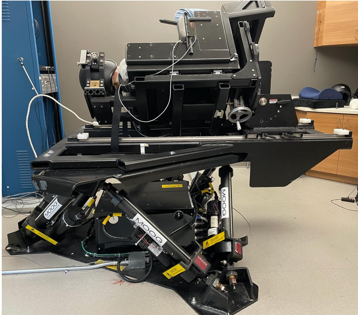
Figure S2. Chair is tilted backward 90 degrees and rotated 45 degrees to the left of supine. Earth vertical LARP rotations were delivered by rotating the subject about an earth vertical axis aligned at the level of the vestibular labyrinths (i.e., head-centered).
